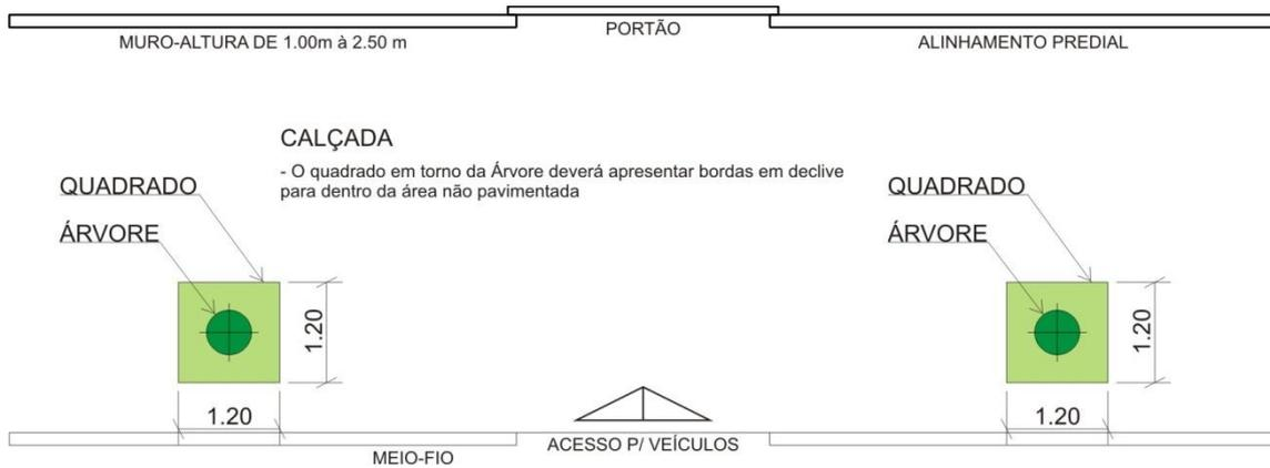
**FIGURA 11: CROQUI ESQUEMÁTICO - CALÇADA PARA ÁREA COMERCIAL**
